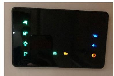
To switch on the panel, simply touch the screen for two seconds.
