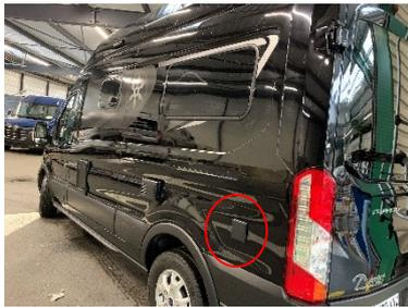
For supplying your vehicle with 230 V, the vehicle must be connected via a standard CEE-coupling outside on the rear left-hand side of the vehicle.
