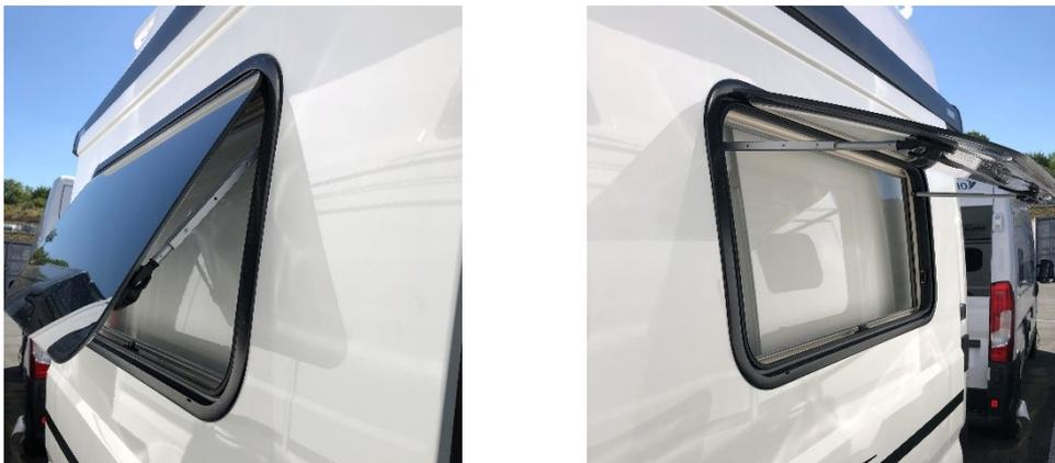
To close the window, open the lever to the stop and then lower it.
