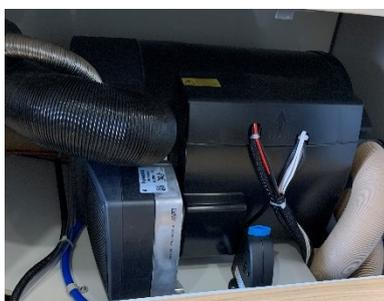
Your vehicle is equipped with a TRUMA D6 heater with integrated boiler, which is located in the rear left-hand box.
