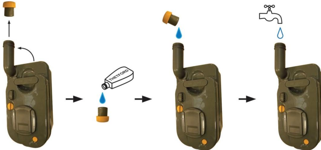
**Note:** In very warm weather or prolonged storage, more WC fluid may have to be used. For best results, use only fluids intended for Thetford toilets. Do not leave any residual amounts in the tank when shutting down for winter.
