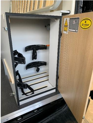
Before shut-down for a longer period of time, it is highly recommended to disconnect the gas cylinders and to store them in a well ventilated place.
